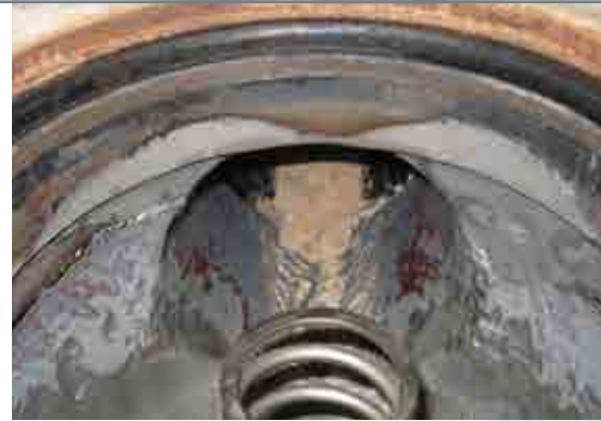
Worn coating exposes metal in <3000 hours.
