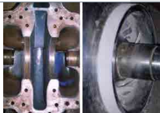
Coated sections of pump.
