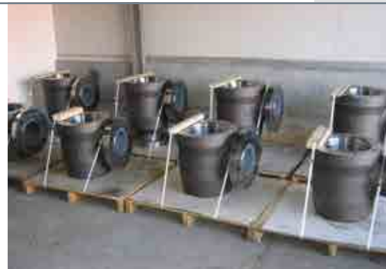
Valves machined and ready for coating.
