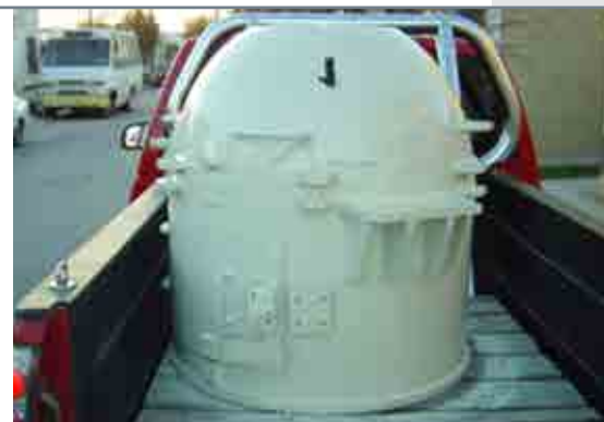
First mill after repair ready for delivery.
