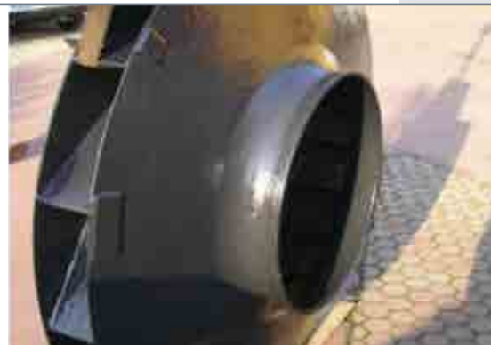
Completed application to 1600 mm fan.
