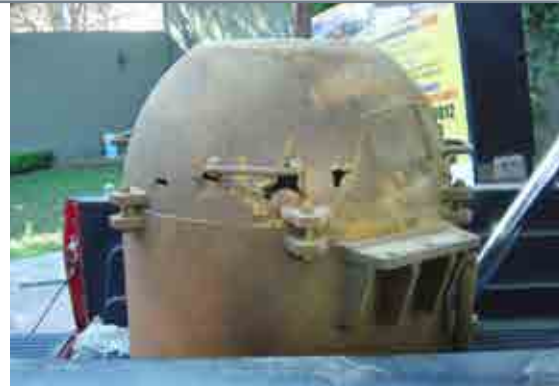
Worn mill after failure of rubber and fiberglass.
